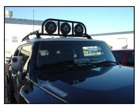
There are several options available for high-power, roof mounted off road lights. One of the best solutions for stock FJ roof racks is the Upper Light Bar from Intense Fabrication. This bar bolts directly to the stock roof rack for easy installation. Available with or without the upper hoop. Starts at \$125.00.
