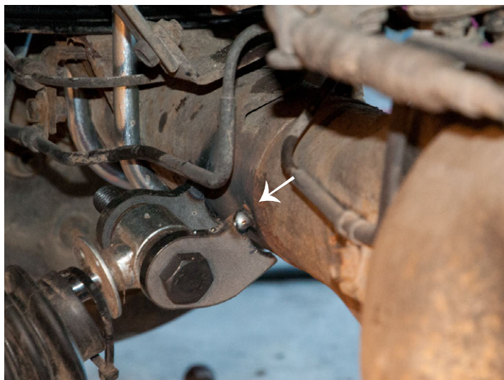
tack weld to hold in place
