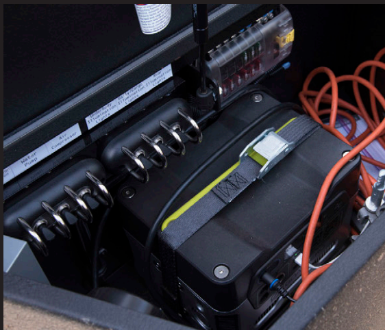
GoalZero Yeti 400 with switches and fuse box sit snug in the smaller battery box.
