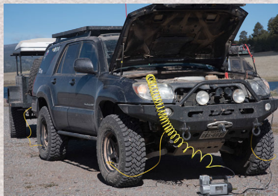
With the 4 whips attached to each air outlet and tire, the portable air compressor is able to inflate the 4 tires evenly.
