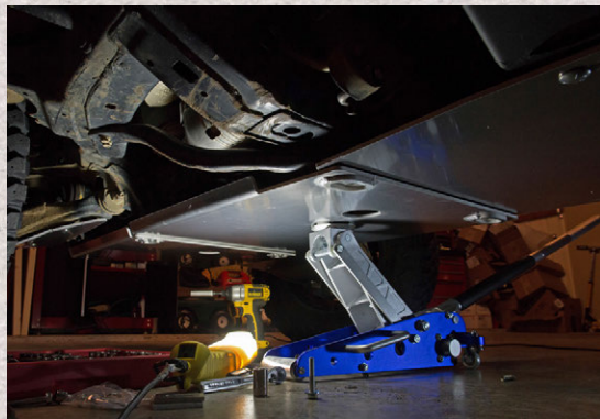
Installation of the complete system went smoothly. The skids overlap each other where the bolts go in. The rearward skid plate terminates at the RCI cross-member.
