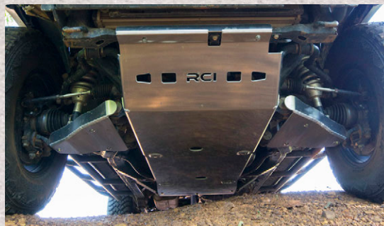
These pretty aluminum skids are fully functional, lighter than steel, and well-designed. They fit perfectly and align as expected.
