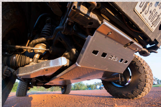
Installation of the complete system went smoothly. The skids overlap each other where the bolts go in. The rearward skid plate terminates at the RCI cross-member.
