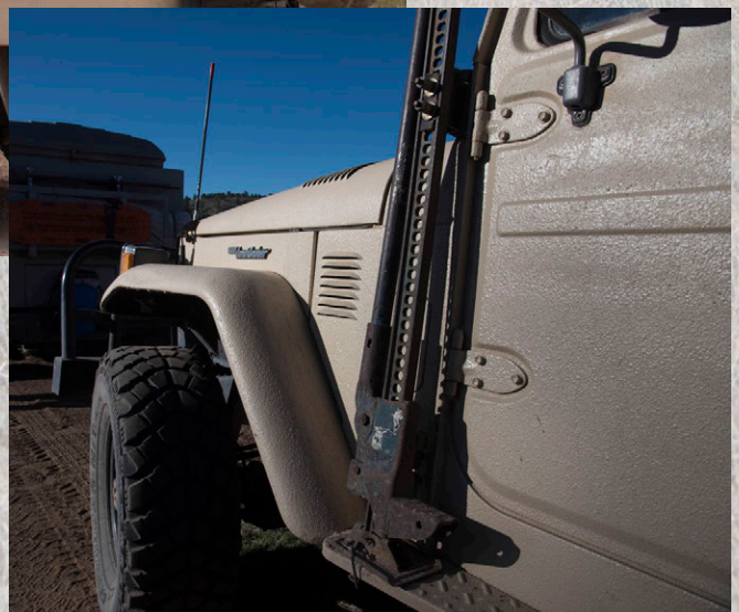
The decades-old Hi-Lift jack is attached with homemade mounting brackets.
