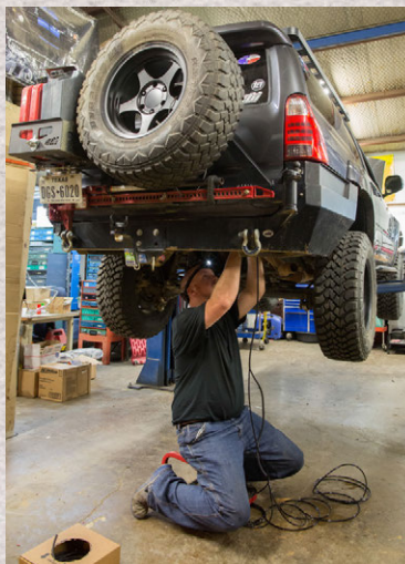
Ben Edwards of Frisbee Automotive, Inc. installs the 2-Way Air lines and outlet ports. The install was clean and structured to prevent failures.
