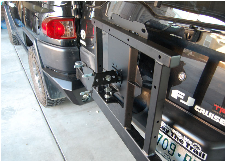
The tire mount is adjustable for different tires/rims and the linkage provides a rattle free mount.
