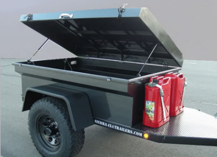
Base trailer with steel wheels, 265-70-R16 BFG AT tires and other options
