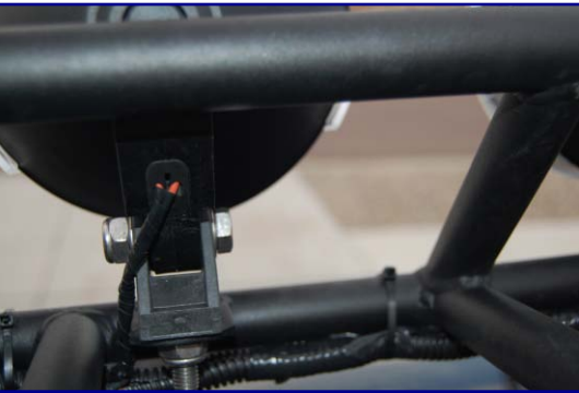
Secured, wrapped, & zip tied wiring
