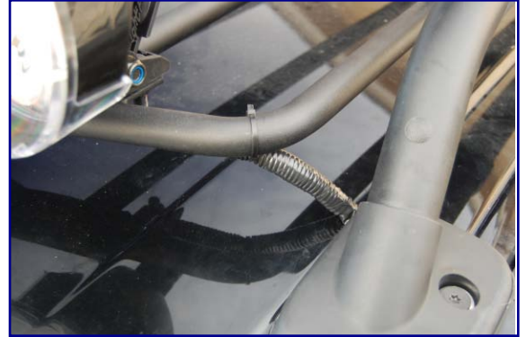
We routed our wires through a hole under the roof rack pad
